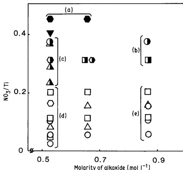
Figure 5 Effects of the amounts of water and acid and of alkoxide molarity on appearance of the gels obtained. (a) Type-3 gel, (b) high density, type-2 gel, (c) low density, type-2 gel, (d) low density, type-1 gel, (e) high density, type-1 gel.
