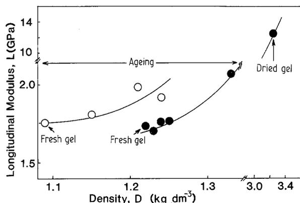
Figure 8 Relation between bulk-density and elastic (longitudinal) modulus of the aged-gels.  $L = DV_L^2$ ,  $V_L$  = sound wave velocity,  $L$  = longitudinal modulus,  $D$  = density. (O) Low-density type-1 gel:  $[H_2O/Ti] = 2.0$ ,  $[NO_3/Ti] = 0.15$ ,  $M = 0.53$  [ $mol\ l^{-1}$ ]; (●) High-density type-2 gel:  $[H_2O/Ti] = 2.0$ ,  $[NO_3/Ti] = 0.38$  and  $M = 0.87$  [ $mol\ l^{-1}$ ].
