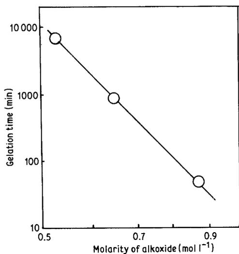
Figure 2 Effect of alkoxide molarity on gelation time.  $\text{H}_2\text{O}/\text{Ti} = 2.0$ ,  $\text{NO}_3/\text{Ti} = 0.15$ .
