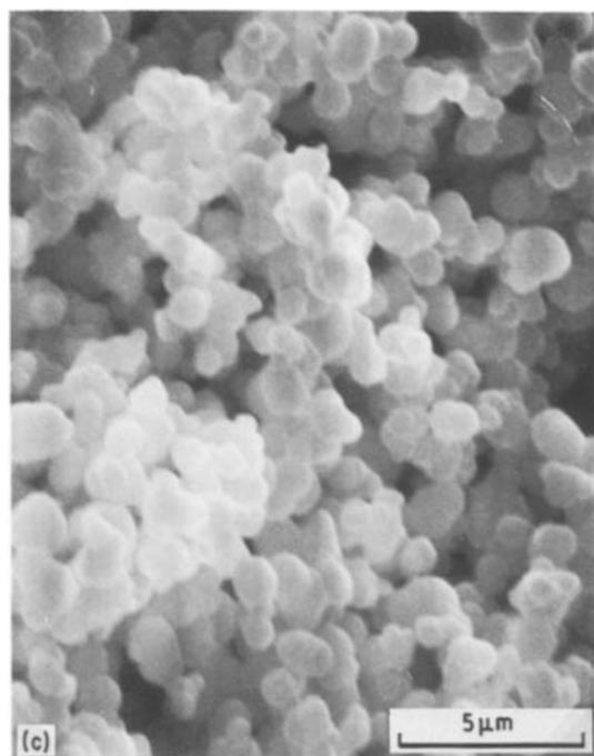
Figure 4 SEM photomicrographs of the fracture surface of dried-gels from (a) type-1, (b) type-2, (c) type-3 gels.
