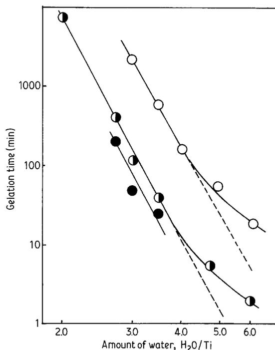
Figure 1 Effect of amount of water on gelation time.  $M = 0.53 \text{ mol l}^{-1}$ , (○)  $\text{NO}_3/\text{Ti} = 0.30$ , (●)  $\text{NO}_3/\text{Ti} = 0.08$ , (◐)  $\text{NO}_3/\text{Ti} = 0.15$ .
