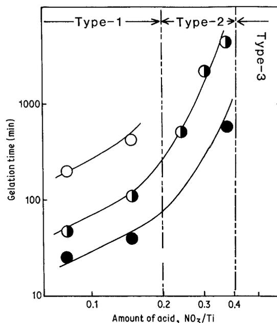
Figure 3 Effects of amount of acid on gelation time and on the appearance of the gel obtained. Type-1, type-2, and type-3 gels correspond to transparent, opaque, and powder-like gels, respectively.  $M = 0.53 \text{ mol l}^{-1}$ , (○)  $\text{H}_2\text{O}/\text{Ti} = 2.7$ , (◐)  $\text{H}_2\text{O}/\text{Ti} = 3.0$ , (●)  $\text{H}_2\text{O}/\text{Ti} = 3.5$ .
