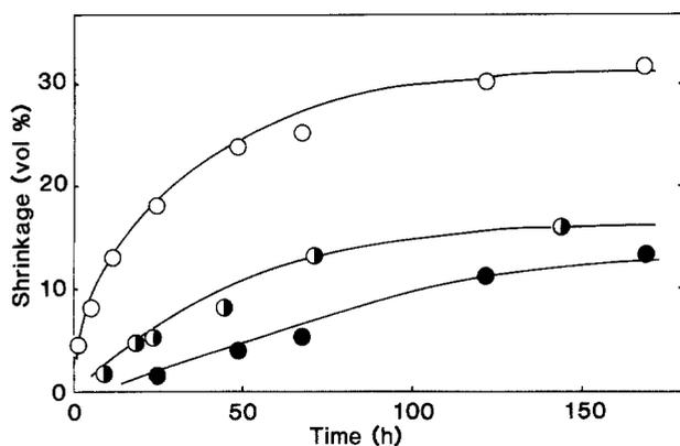
Figure 7 Effect of amount of acid on gel-shrinkage during ageing at 70°C.  $H_2O/Ti = 2.0$ ,  $M = 0.53$  ( $mol\ l^{-1}$ ), (O)  $NO_3/Ti = 0.38$  (type-2), (◐)  $NO_3/Ti = 0.15$  (type-1), (●)  $NO_3/Ti = 0.08$  (type-1).
