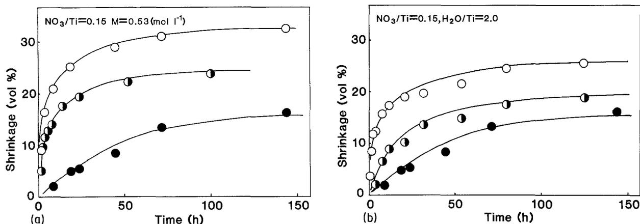
Figure 6 Effects of (a) amount of water ((○) H<sub>2</sub>O/Ti = 3.0, (●) H<sub>2</sub>O/Ti = 2.7, (●) H<sub>2</sub>O/Ti = 2.0) and (b) alkoxide molarity ((○)  $M = 0.87 \text{ mol l}^{-1}$ , high density gel, (●)  $M = 0.66 \text{ mol l}^{-1}$ , (●)  $M = 0.53 \text{ mol l}^{-1}$ , low density gel) on gel-shrinkage during ageing at 70°C.
